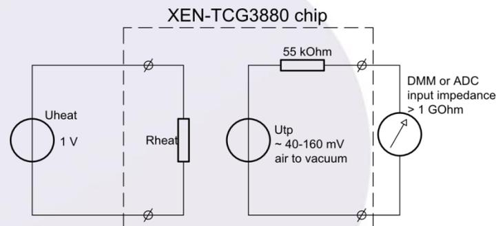
**Figure 2:** Constant voltage biasing of the XEN-TCG3880 for vacuum measurement.
