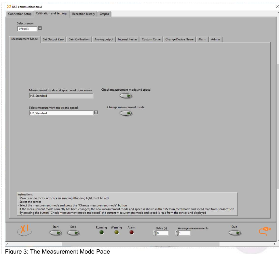
Figure 3: The Measurement Mode Page
