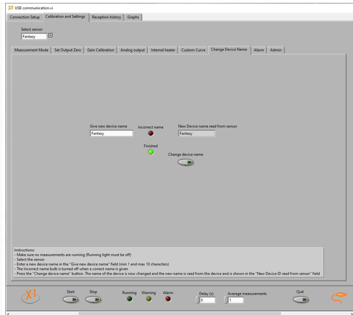
Figure 10: The Change name device ID page, which can be used to change the device ID of the XEN-5320
