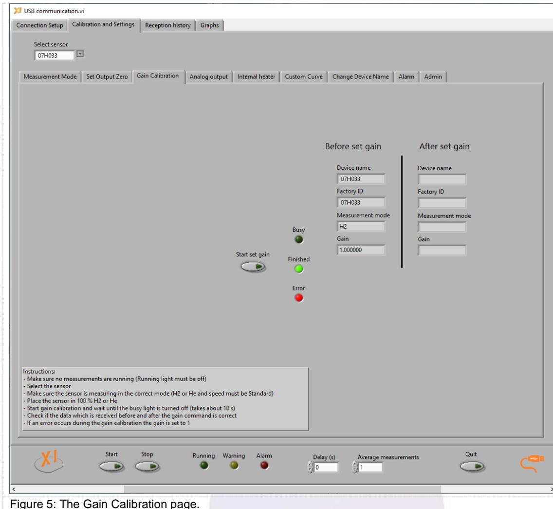
Figure 5: The Gain Calibration page.
