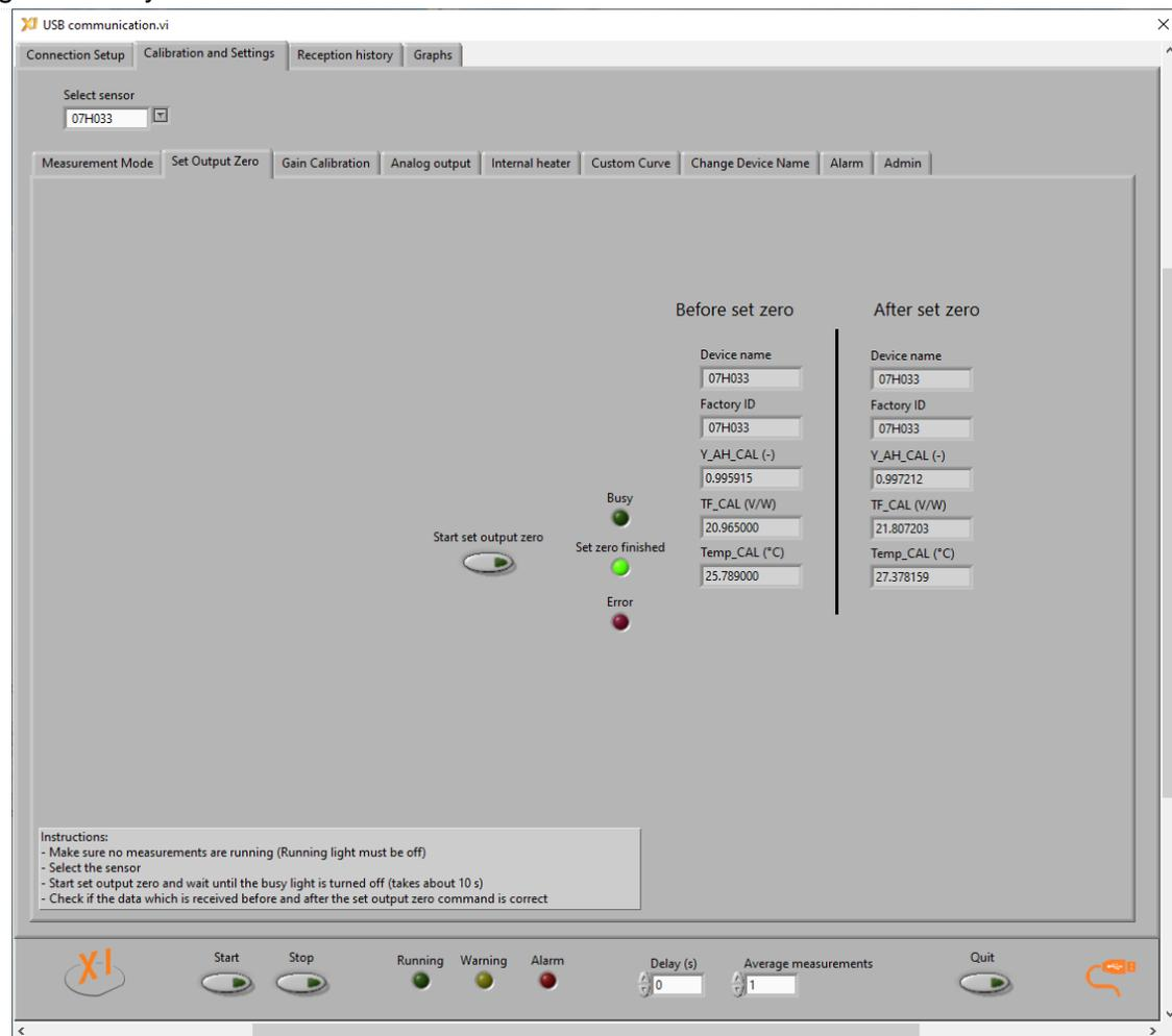
Figure 4: The Start output zero Page, with data of the device before and after zeroing.
